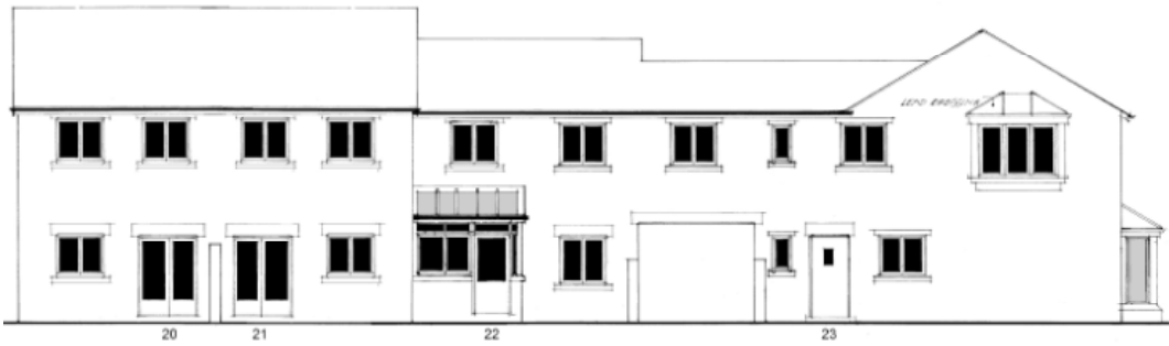
Rear elevation for units 20 – 23 showing large south facing windows maximising passive solar gain
