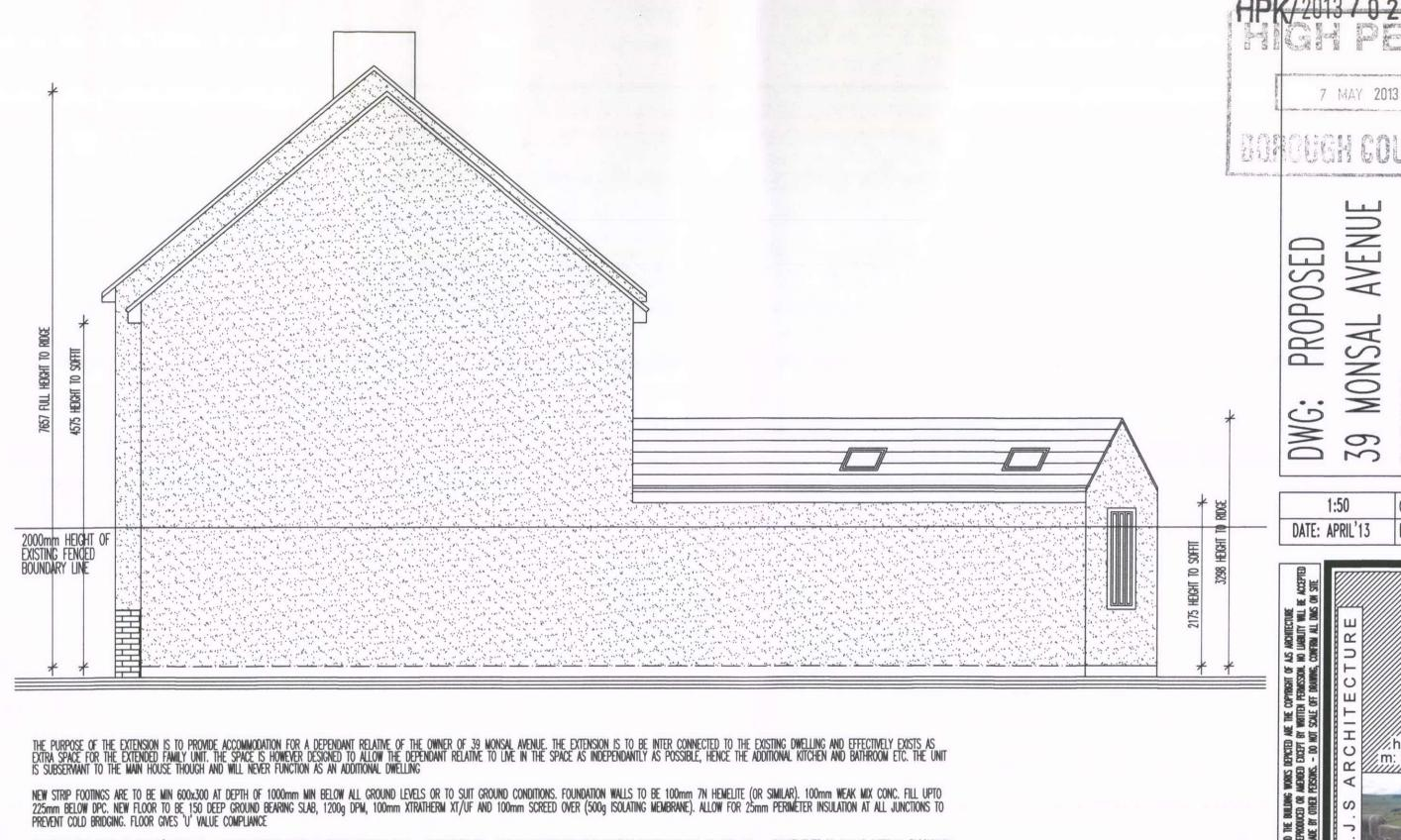
NEW STRUCTURE IS TO BE 300 0/A WITH 100mm OUTER DASHED BLOCK TO MATCH EXISTING, 100mm CAVITY WITH 60mm XTRATHERM POLYISO XT INSULATION MAINTAINING MIN AIR GAP. 100mm 7N HEMELITE OR SIMILAR INTERNAL BLOCKWORK WITH 12.5mm PBD ON DABS. STRUCTURE GIVES U VALUE IN COMPLIANCE WITH BUILDING REGS.
