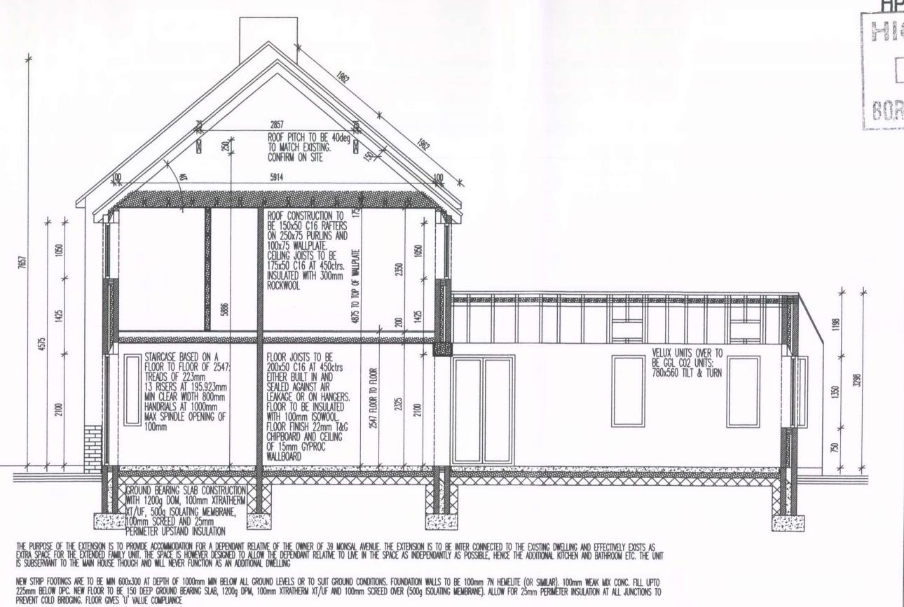
NEW STRUCTURE IS TO BE 300 O/A WITH 100mm OUTER DASHED BLOCK TO MATCH EXISTING, 100mm CAVITY WITH 60mm XTRATHERN POLYISO XT INSULATION MAINTAINING NIN AIR GAP. 100mm 7N HEMELITE OR SIMILAR INTERNAL BLOCKWORK WITH 12.5mm PBD ON DABS. STRUCTURE CIVES U VALUE IN COMPLIANCE WITH BUILDING REGS.
