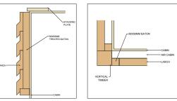
CLADDING DETAIL CLADDING DETAIL SECTION **CORNER DETAIL**
