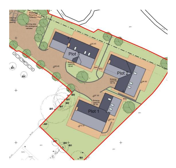
The proposed 3 no detached dwellings continue the relatively low density of development evidenced on Church Lane in a 'cluster' site layout, wrapping around the end of the access road and forming the impression of a courtyard, at levels to suit the existing topography of the site.
