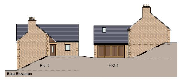
The properties are designed to be step down/up the existing topography of the site. Plot 1 is two storey to the front, single storey to the rear, whilst plots 2 and 3 are single storey to the front and step down into the valley to be 2 storey at the rear.
