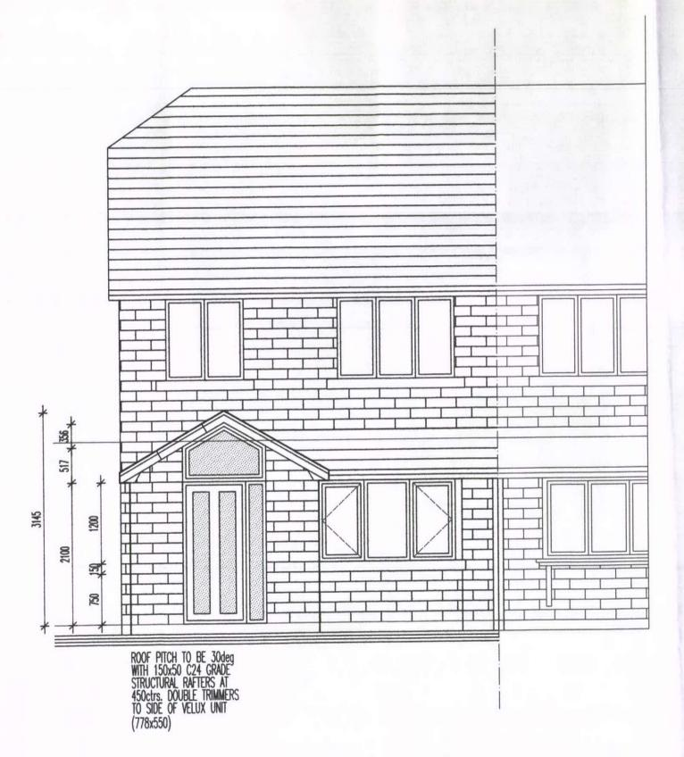
THE PROPOSAL RELATES TO THE CONSTRUCTION OF NEW PORCH EXTENSION AND REVISED BAY CONSTRUCTION TO ALLOW FOR A COMPLETE BAY WITH CAVITY CONSTRUCTION BELOW AND NEW FLOOR AS PART OF THE LOUNGE AREA
