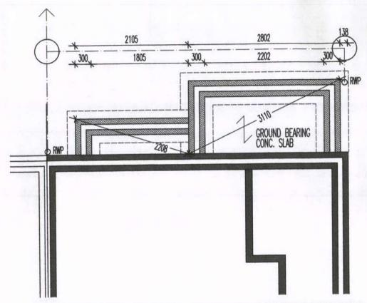
FOOTINGS TO NEW EXTERNAL WALL 600x300mm MIN THICK. DEPTH OF FOUNDATIONS TO SUIT GROUND CONDITIONS. — MIN 600mm. AGREE ALL DETAILS FOLLOWING FURTHER SITE INVESTIGATION.
