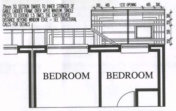
C24 GRADE 150x50 RAFTERS AT 450ctrs SAT ON 100x75 TIMBER WALLPLATE, BEDDED IN MORTAR. ALL TIES, RUNNERS AND DIAGONAL BRACING TO BE 100x25mm TWICE NAILED TO EACH RAFTER WITH 3.35x75nn LONG GALV WIRE.
