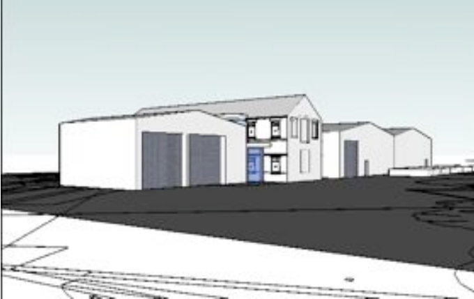
Fig.5 Image showing the Proposed portal frame being pulled back from the front edge of the existing warehouse allowing the stone building to be viewed and respected as well as provided a clear entrance.
