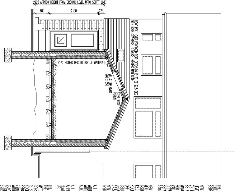
THE PROPOSAL RELATES TO THE CONSTRUCTION OF NEW SINGLE STOREY EXTENSION OVER THE EXISTING FRONT PORCH TO PROVIDE AN EXTENDED BEDROOM. REAR EXTENSION AND AREA TO THE SMALL F
