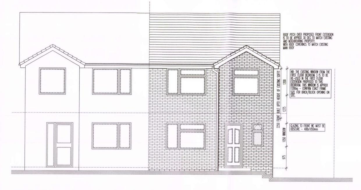
THE PROPOSAL RELATES TO THE CONSTRUCTION OF NEW SINGLE STOREY REAR EXTENSION AND AN EXTENSION OVER THE EXISTING FRONT PORCH TO PROVIDE AN EXTENDED AREA TO THE SMALL FRONT BEDROOM.
