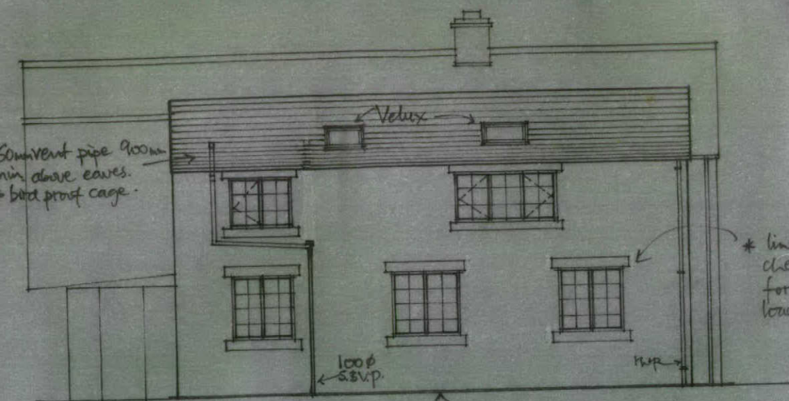
NORTH WEST ELEVATION.
