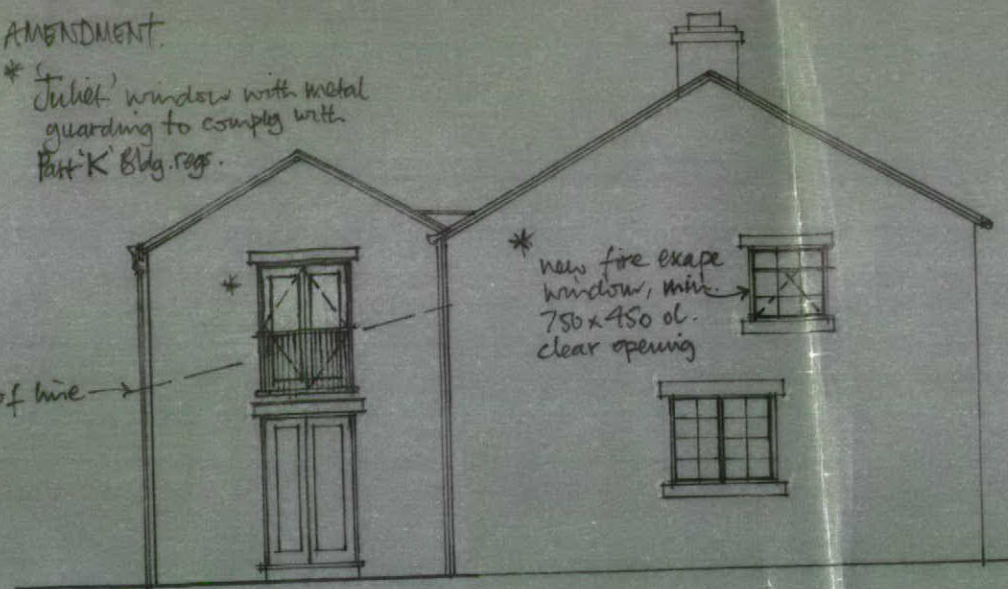
SOUTH WEST ELEVATION.
