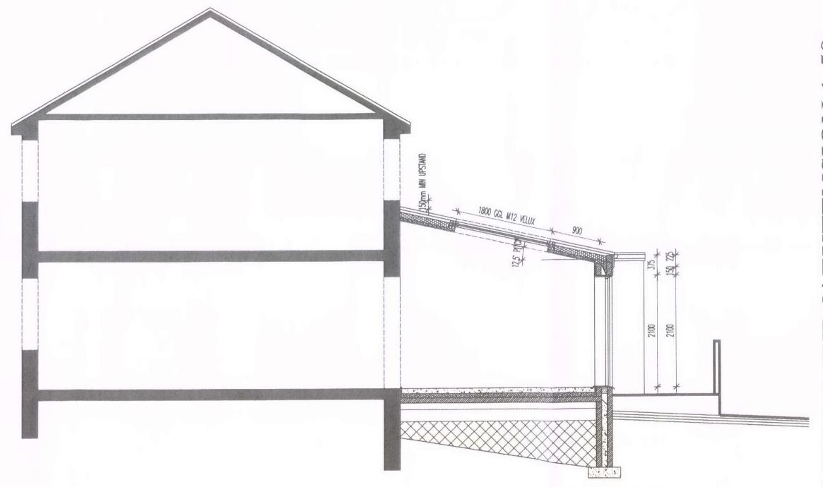
PROPOSAL IS TO DEMOLISH THE EXISTING UPVC CONSERVATORY TO THE REAR AND CONSTRUCT A NEW SINGLE STOREY EXTENSION THAT WILL ADJOIN THE EXISTING ANNEX BUILDING THAT IS TO REMAIN TO THE SIDE.
