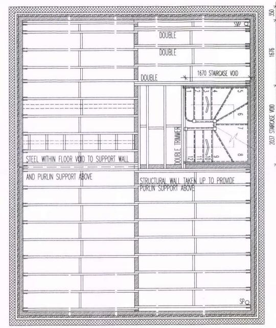
FLOOR JOISTS AT FIRST FLOOR ARE TO BE 200x50 C24 GRADE STRUCTURAL TIMBER AT 450mm ctrs. ALL JOISTS ARE TO BE ON PROPRIETARY JOIST HANGERS. ALLOW FOR STRAPS AT 1200mm ctrs OVER THE 3 JOISTS ADJACENT TO THE EXTERNAL WALL.
