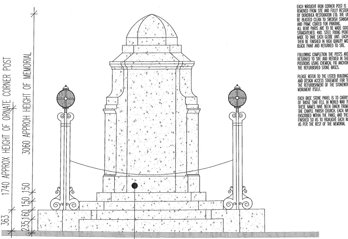
THE GLOBE LIGHTING INDICATED TO THE TOP OF EACH CORNER POST IS FOR ILLUSTRATIVE PURPOSES ONLY - DOROTHEA RESTORATION LTD ARE TO SUPPLY design details under separate cover.
