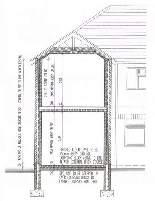
CONCRETE STRIP MIN. 600 x 200min. THICK TO CAVITY WALLS & MIN. 450 x 200 THICK TO 1/2 BRICK / LOADBEARING WALLS TO SITE SPECIFIC ENGINEERS DETAILS OR 425 WIDE CONCRETE TRENCH FILL FINISHED AT LEAST 150 BELOW G.L IN CLAY SOIL NOT AFFECTED BY TREE GROWTH OR REMOVAL DEPTH OF FOUNDATIONS TO SUIT GROUND CONDITIONS TO FIRM BED & TO APPROVAL OF BUILDING INSPECTOR. N.B. PRECAUTION AGAINST ROOT DAMAGE TO BE AGREED ON SITE WITH BUILDING INSPECTOR AND TO NHBC STANDARDS — CHAPTER 4.2.
