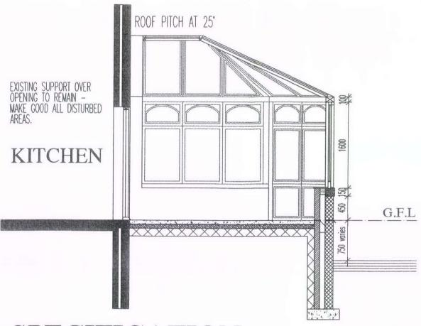
EXISTING REAR WINDOW OFF KITCHEN TO BE OPENED UP TO FORM A 1200mm FRENCH DOOR OPENING TO LEAD INTO NEW CONSERVATORY.
